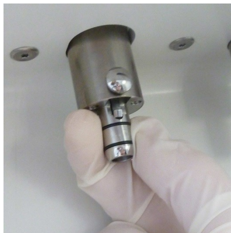
Figure 29: O-ring joints of E-type connector
