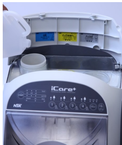
Figure 13: Filling the Oil tank of iCare+ device
