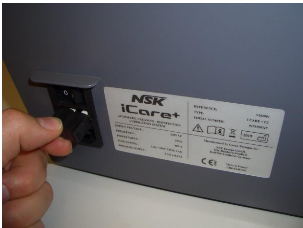
Figure 30: Fuse box of iCare+ device
