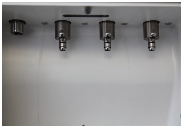
Figure 18: iCare+ version 1 with 1 air turbine and 3 E-type connectors
