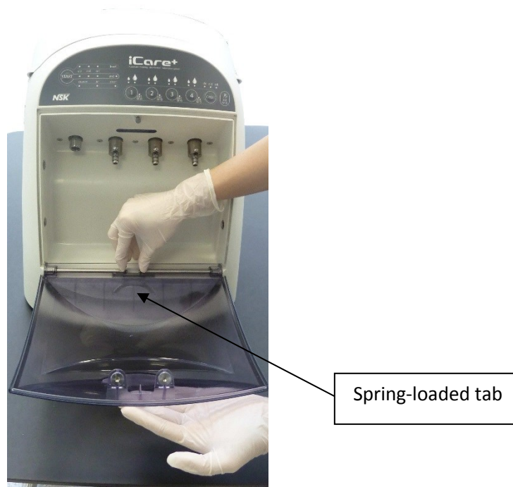
Figure 24: Access to the treatment chamber of iCare+ device
